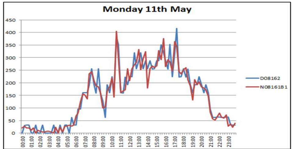
The validation of the SCOOT link was carried out in the same way it would be for a link using an inductive loop. The parameters entered were unaffected by the detector type, with the Saturation Occupancy (STOC / SATO) value being within the expected range for a single lane junction approach.
